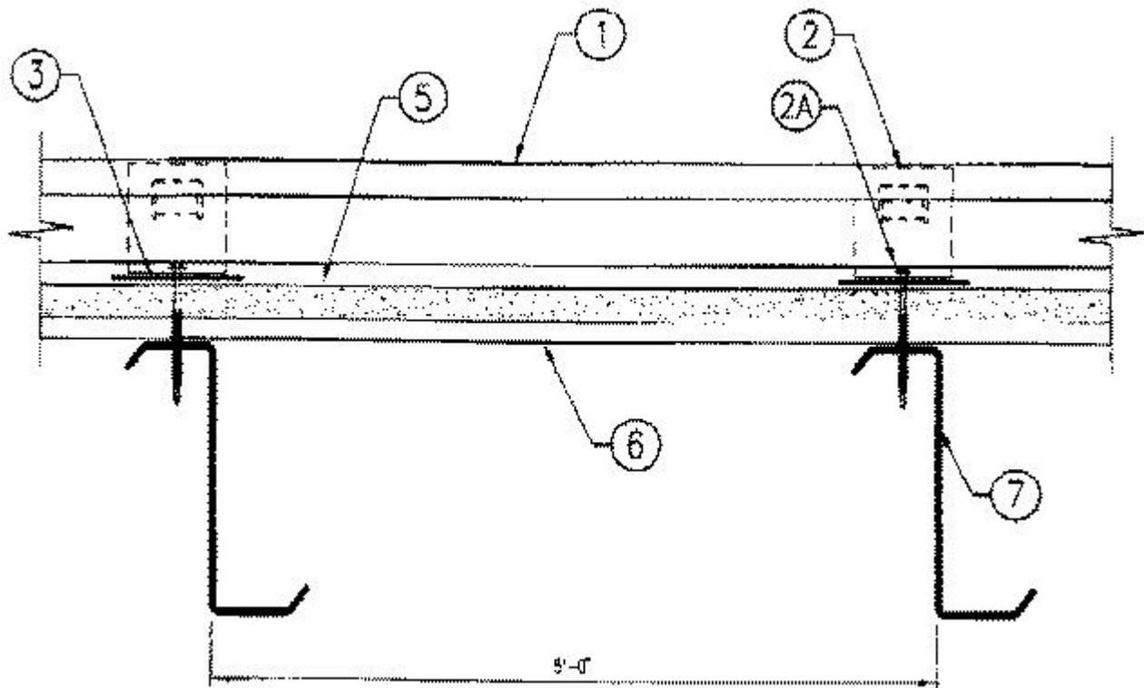
1. **Metal Roof Deck Panels\*** — No. 24 MSG min coated steel. Panels continuous over two or more spans. Endlaps to occur adjacent to purlin with panels overlapped 3 in. A bead of sealant may be used at panel end joints.
