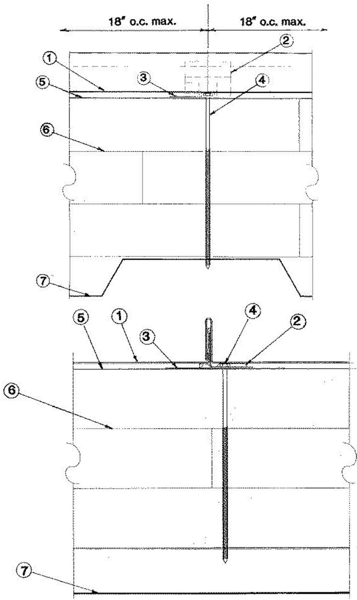
1. **Metal Roof Deck Panels\*** — No. 24 MSG min coated steel, 20 in. wide or 12 in. wide, 1-1/2 in. high at female side rib. Panels continuous over three or more clips with no end laps. A bead of sealant may be used at panel side joints.
