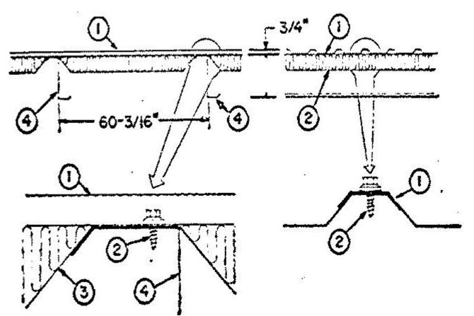
1. **Metal Roof Deck Panels\*** — No. 26 MSG min gauge coated steel. Panels continuous over two or more spans. End laps to occur over purlins with panels overlapped 6 in. with lap beginning 1 in. from edge of purlin flange and extending across purlin. A bead of sealant may be used at panel end and side laps.
