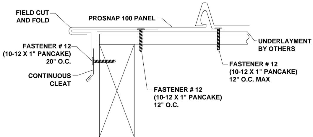
Figure 6: Alternative Rake/Gable Flashing Detail
