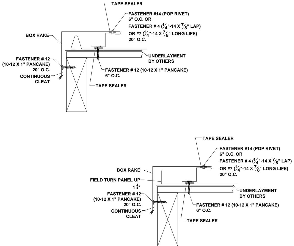
Figure 7: Box Rake/Gable Flashing Detail
