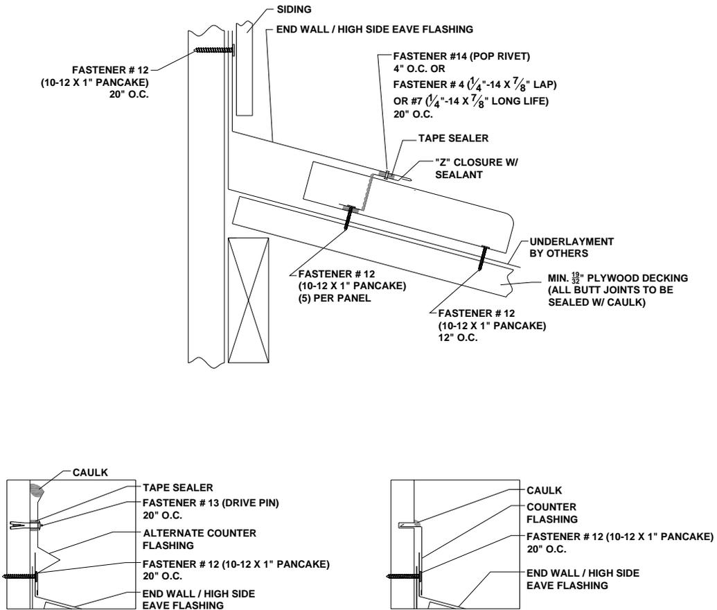
Figure 9: Fixed Endwall / Parapet High Side Eave Detail
