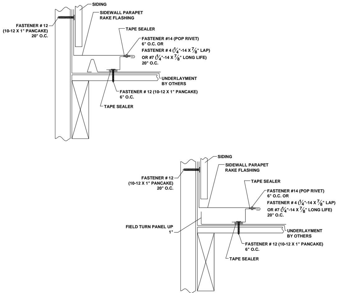
Figure 8: Sidewall / Parapet Fixed Rake Flashing Detail
