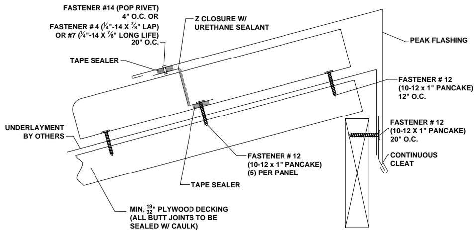
Figure 5: Fixed Peak Flashing Detail
