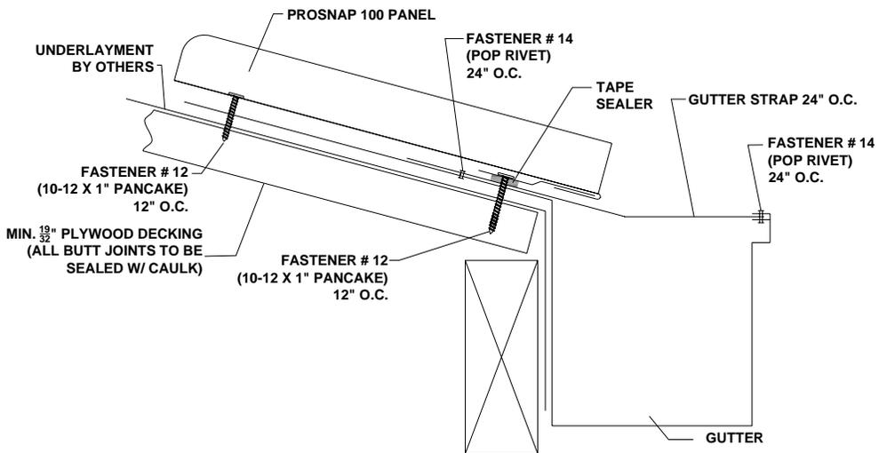
Figure 4: Gutter Detail
